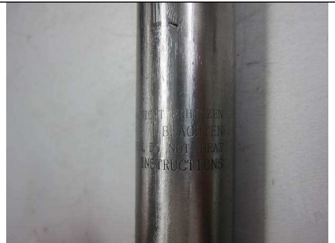
Pic.6: Gas spring marking
