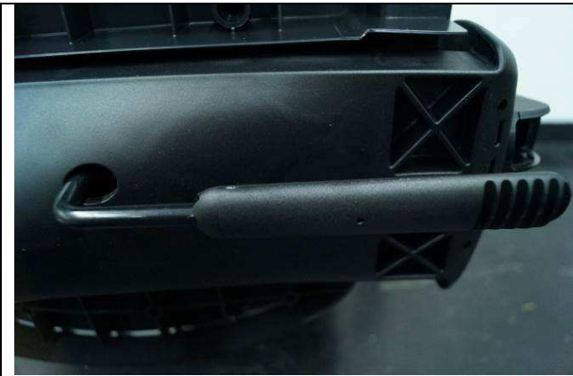
Pic.5: Seat height adjust lever
