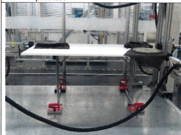
Pic.9: Horizontal durability test
